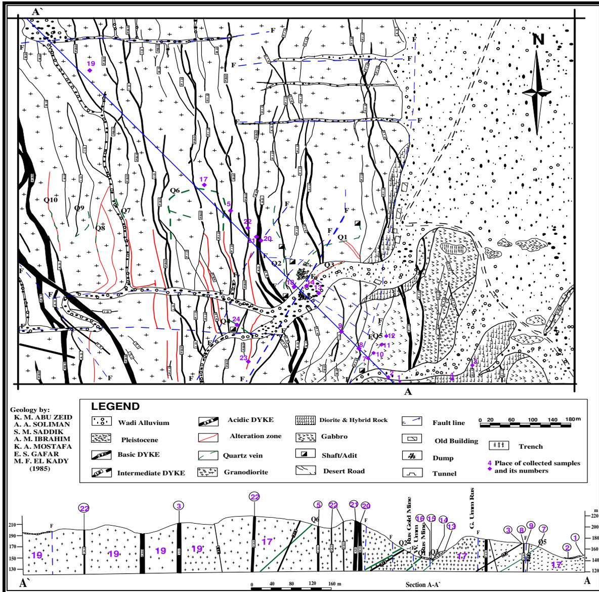
Figure 2: Geological map of the Umm Rus gold deposits (Abu Zeid et al, 1985). -samples for this study were collected along geological cross-section A-A`
