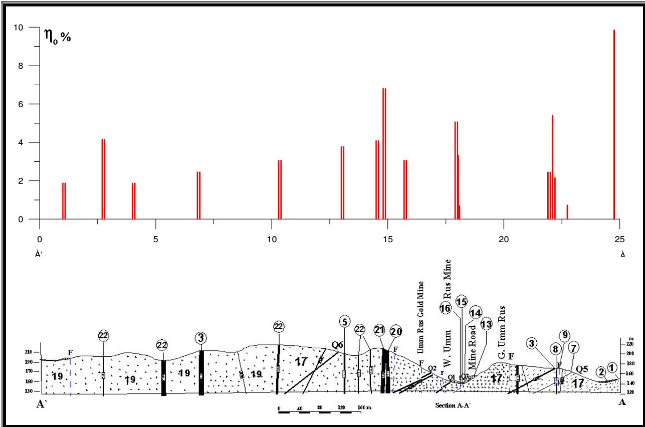
**Figure 3:** Geological cross section A-A` across the Umm Rus gold deposits with the value of the stationary polarizability measured for the rock samples are plotted against the concerned sample location. .
