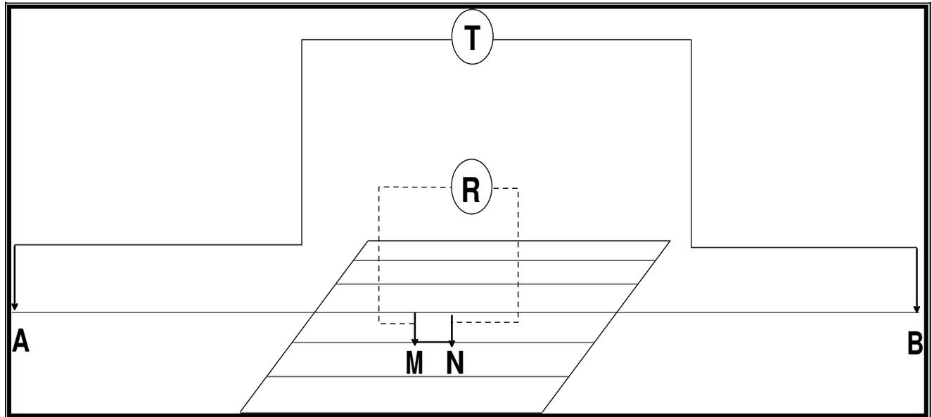
**Figure 4:** Scheme of the middle gradient array used for field measurements.
