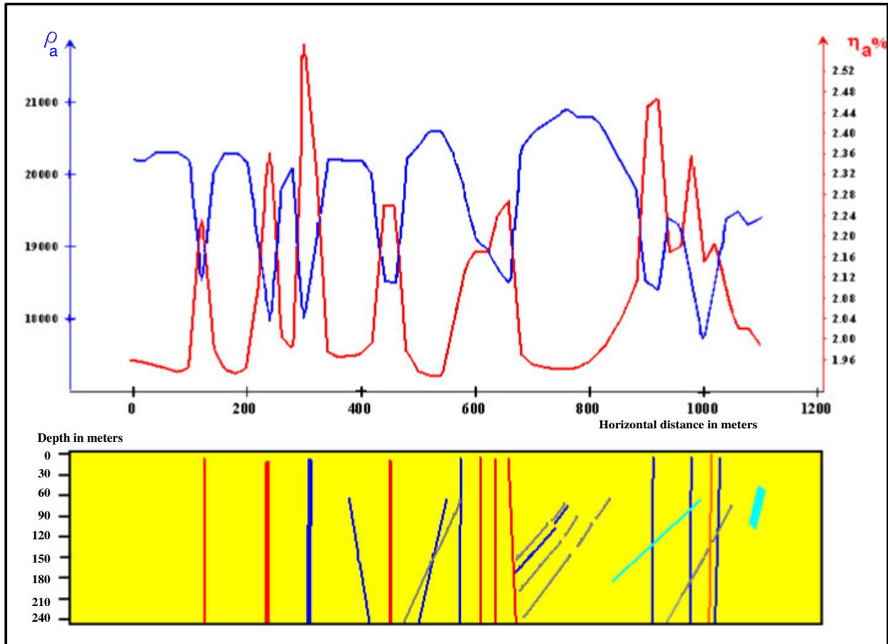
**Figure 5:** Resistivity and polarizability values plotted against the samples along geological cross section (A-A').
