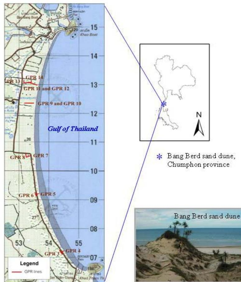
**Figure 1.** Bang Berd sand dune is located at Pathio district, Chumphon province, the western coast of the Gulf of Thailand. GPR lines survey was conducted along – transects oriented parallel and perpendicular to the dune’s downwind axis, 12 lines (total length 1,510 m).
