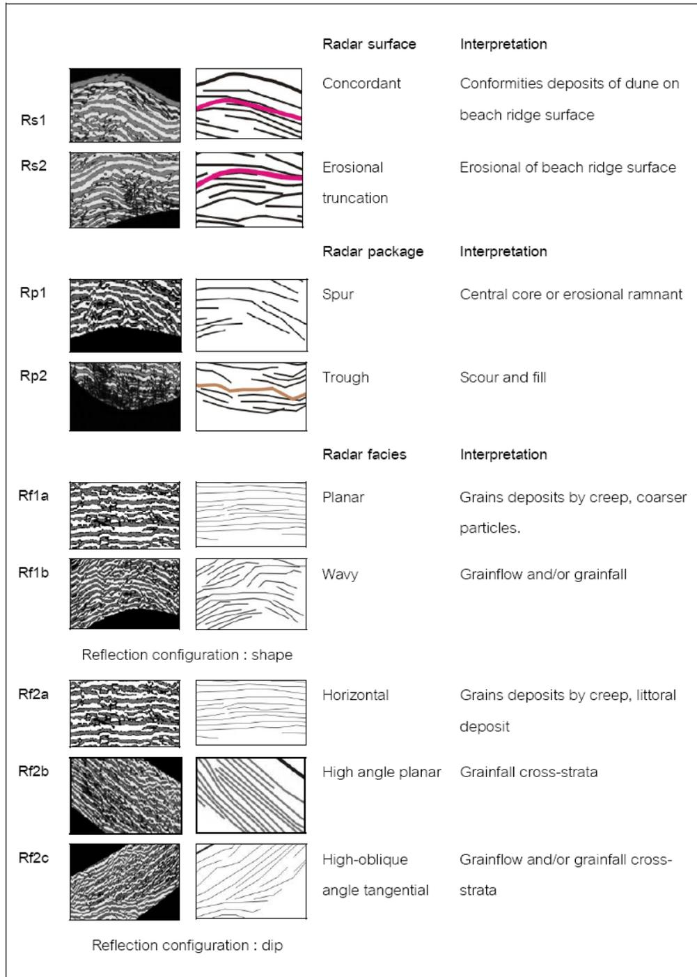
**Figure 6.** Main feature from the radar profiles can be classified into 2 radar surfaces. They are concordant (Rs1) and erosional truncation (Rs2). Two radar packages are spur (Rp1) and trough (Rp2) and five radar facies included a planar (Rf1a), wavy (Rf1b), horizontal (Rf2a), High angel planar (Rf2b) and high-oblique angel tangential (Rf3b).
