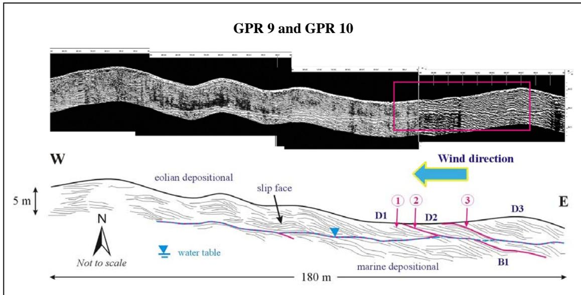
**Figure 4.** GPR 9 and GPR 10 were conducted along – transects oriented parallel to the dune’s downwind axis, showing the contact between three different dune generations (unit D1, D2 and D3) by third order bounding surface (mark 1, 2 and 3 in picture). Direction of wind blown was expected from the east to the west.
