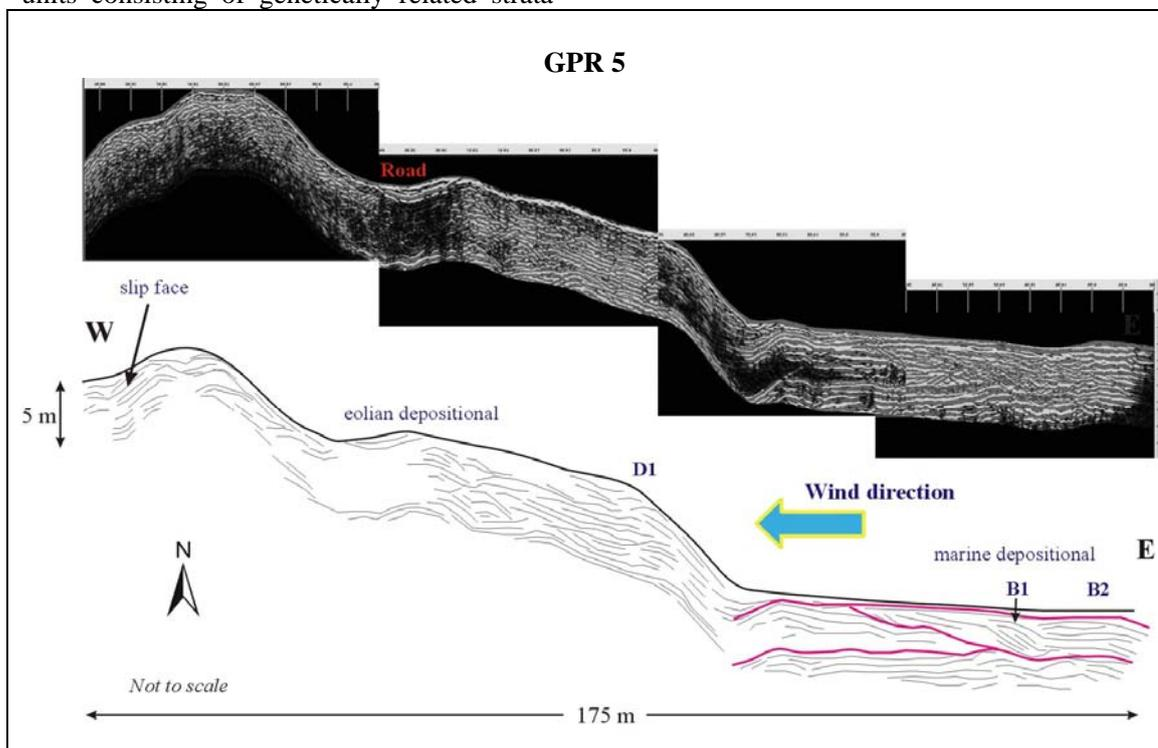
**Figure 3.** GPR 5 was conducted along – transects oriented parallel to the dune’s downwind axis. The characteristics of marine sediment are beach ridge (unit B1) generally dip seaward and littoral deposit (unit B2) horizontal layer. Slip-faces of dune represent the probable direction of wind blown from the east to the west.
