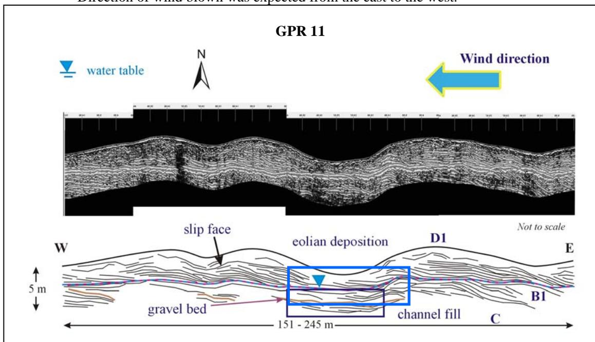
**Figure 5.** GPR 11 was conducted with orientation parallel to the dune’s downwind axis, showing a trough shape underlie beach ridges represent to channel fill deposit (unit C). Direction of wind blown was expected from the east to the west.
