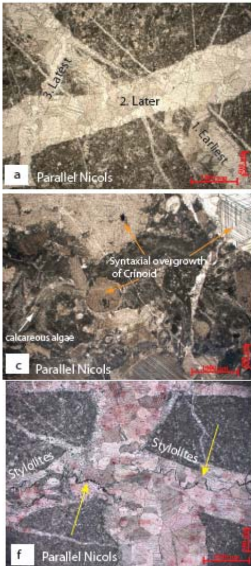
Figure 4. a) Three stages of development in a breccia zone (S7); (c) & (d): Crinoidal packstone with calcareous algae, syntaxial overgrowth of echinoderm in breccia zone (S11); (f): Calcite crystals are truncated by stylolites + the displacement of calcite veins in the earlier calcite veins shows the different stages in non breccia zones (S2).
