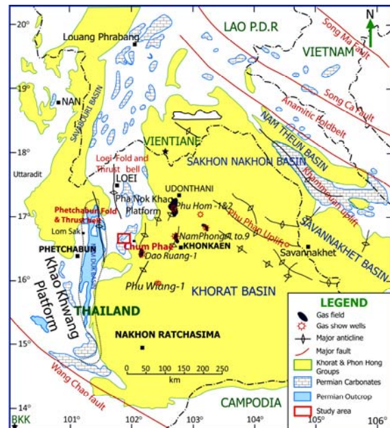
Figure 1. Surface geological elements of the Khorat Plateau Basin, hydrocarbon discoveries and the study area indicated by red rectangle (after Lovatt, Smith & Stokes, 1997; Metcalfe and Sone, 2008).
