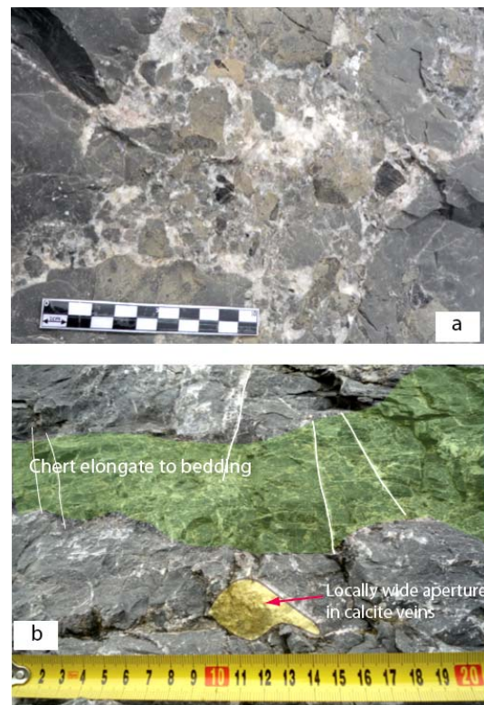
Figure 3. Matrix and calcite veins in (a) breccia zone, (b): in non breccia zones.
